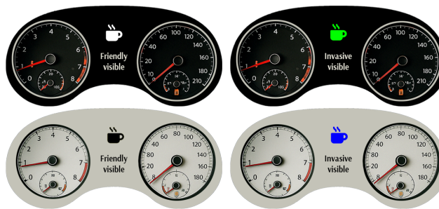
Fig. 4. Example of alert colors for dark and light modes in the car interface for Friendly and Visible (Left) and Rapid Attention Capture (Right) scenarios.
